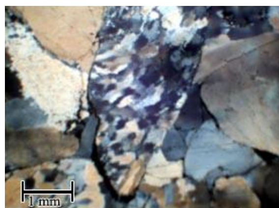
Figure 7: Less Matrix and Cement with Microstylolitic Contracts, Note the Poly Crystalline Quartz
